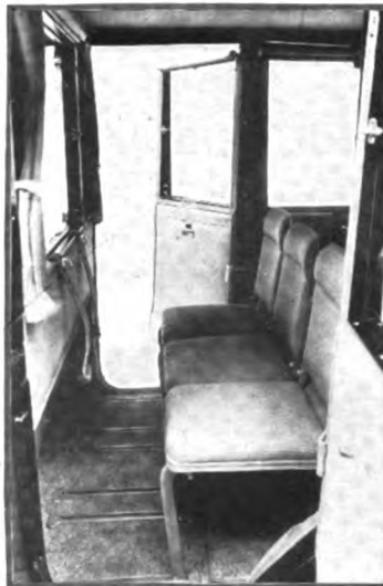
COLE'S-THREE DISSAPPEARING SEATS IN BERLINE
